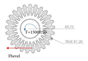
Note: while normally the key of the bevel gear would fail before the tooth, my bevel gear part is modeled as an extruded shaft and is very well supported, so the tooth would definitely fail before the shaft failed, allowing me to do a simpler FBD and FEA analysis. This is true for both the initial and the redesigned bevel gear. In actual manufacturing, a different manner of attaching the bevel gear to the shaft would have to be considered. A square drive shaft might be a good idea, for instance.
