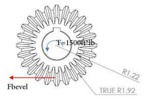
After my FEA analysis of the initial bevel gear (see below) failed before my shear pin did, I redesigned to have a larger bevel gear, allowing the load on the tooth to be smaller, given the increased radius to transmit torque, and allowing the bevel gear's individual teeth to be larger and able to support more load.
