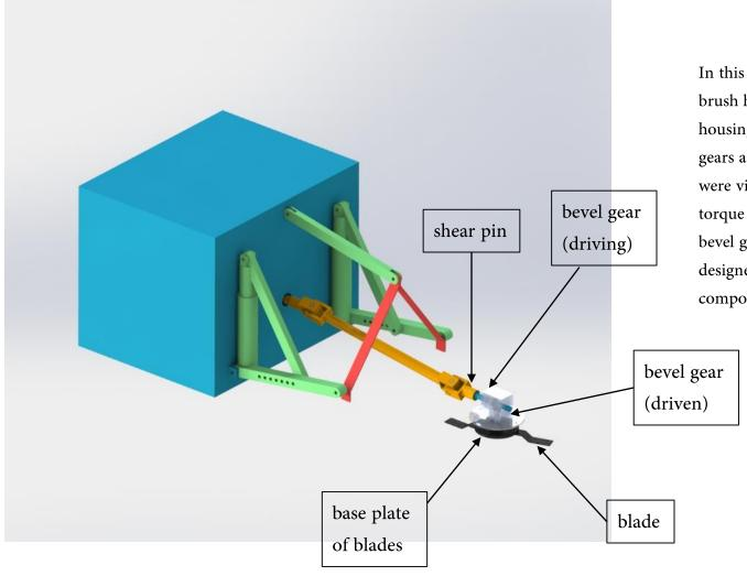
In this view, I hid the body of the brush hog and made the bevel gear housing transparent so the bevel gears and the blade subassembly were visible. A shear pin transmits torque from the PTO shaft to the bevel gear subassembly, and is designed to fail before any other component.
