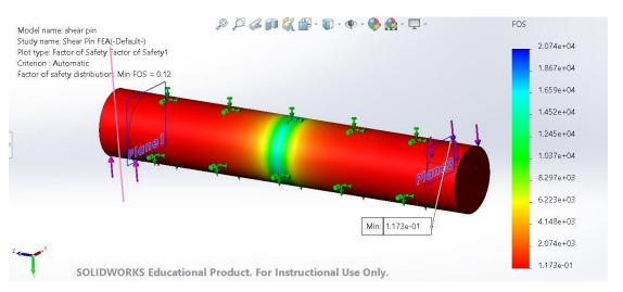
The shear pin's lowest factor of safety ended up being 0.12. It definitely fails.
