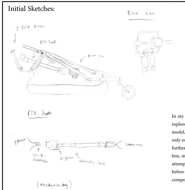
In my initial sketching and ideation phase, I explored different shapes of my brush hog model, eventually settling on using one with only one pair of blades. I then went into further depth sketching out my bevel gear box, my 3-point hitch, and my PTO shaft, attempting to understand these mechanisms before settling on dimensions and specific components.
