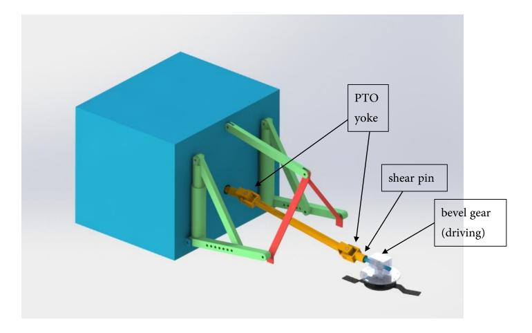
On these parts, I applied a torque (1500 ft lbs) that would cause any of my most heavily loaded parts to fail, with the intension of analyzing which parts failed more easily, so I could see which part would fail first. The hope was that the shear pin would fail before any other component of the transmission, so that it could be replaced without the rest of the transmission being destroyed.
