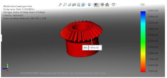
The initial design of my bevel gear had a factor of safety of 0.08, indicating that it would fail before my shear pin, assuming the full load was taken by one tooth. To prevent it failing, I redesigned to use a larger bevel gear.
