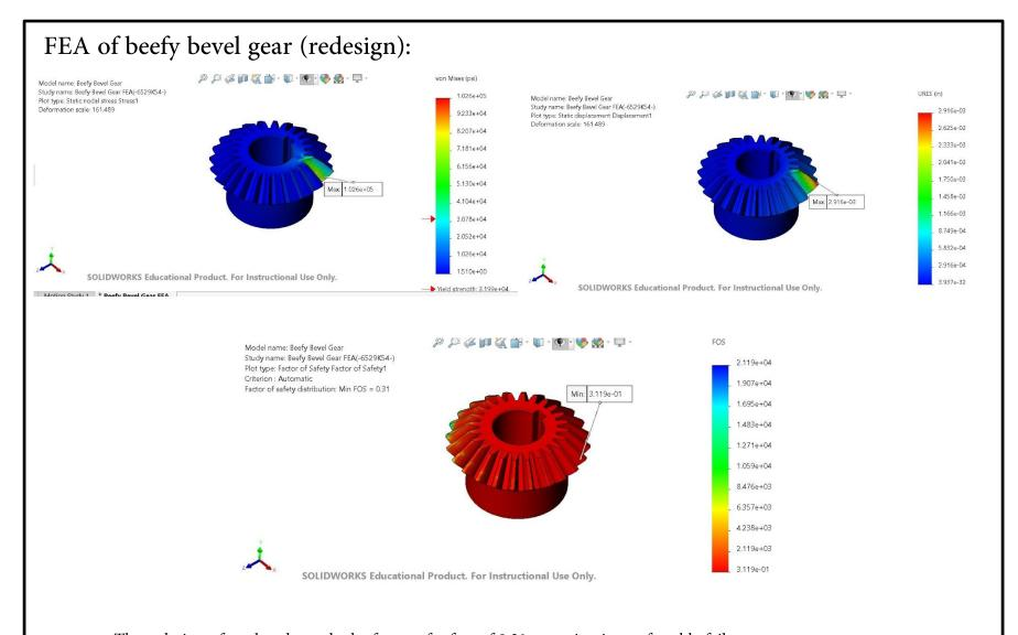
The redesign of my bevel gear had a factor of safety of 0.31, meaning it comfortable fails after the shear pin does. However, an even larger bevel gear might be considered for actual design.
