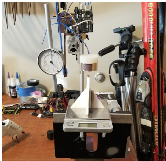
Figure 1: Our measurement setup. We connected the magnet to a scale and moved the scale up and down to measure force at different distances.
